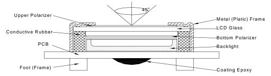
2. View Angle: with in 45° around perpendicular line.
